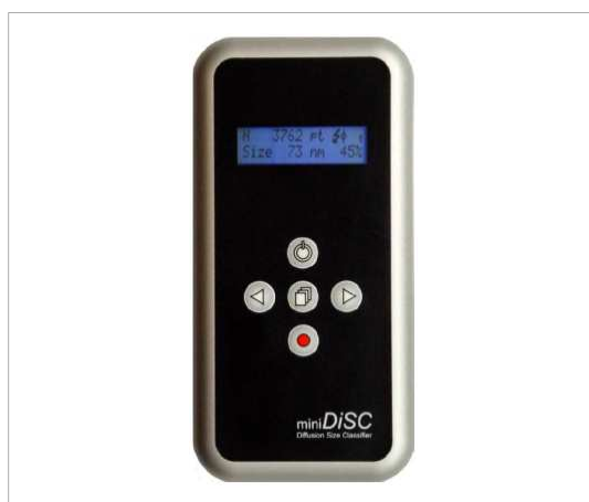
Fig 42: MiniDiSC handheld particle counter
